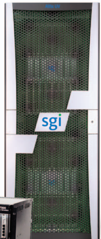
Real-time digital simulator using SGI super computer
