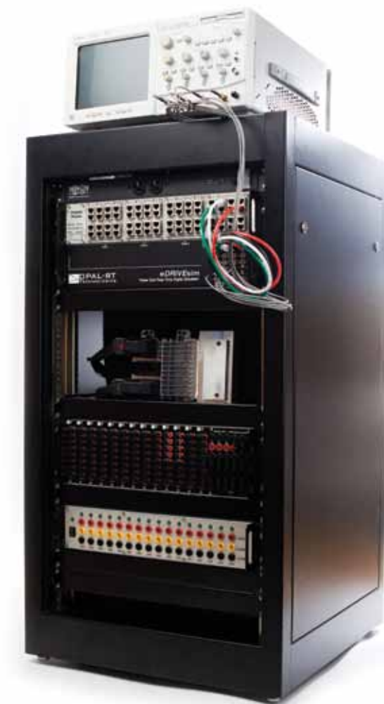
Typical eDRIVEsim™ enclosure with accessories such as Fault Insertion Units (FIUs), Break Out Boxes (BOB) and Mapping Boxes
